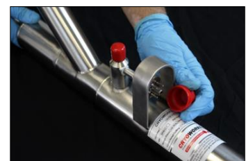
Picture 22 – Evacuation Port
