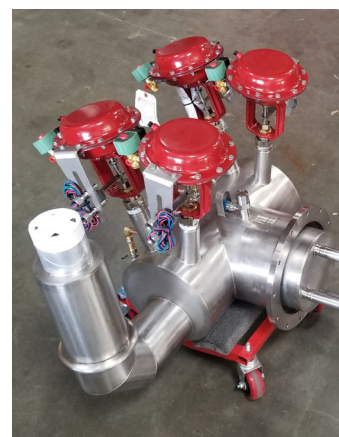
Vacuum Chamber Valve Box Manifold
