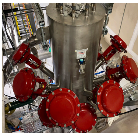
Vacuum Chamber Vent Manifold
