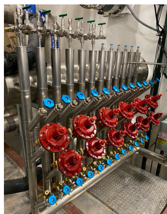
Vacuum Chamber Inlet Manifold
