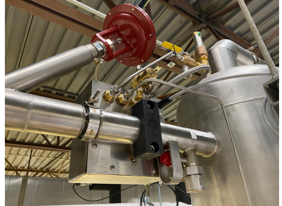
Production ready MBE system with liquid level controller and feed control valve
