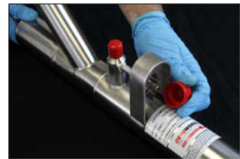
Picture 18 – Evacuation Port
