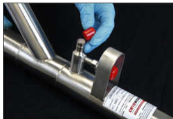
Picture 17 – Evacuation Port
